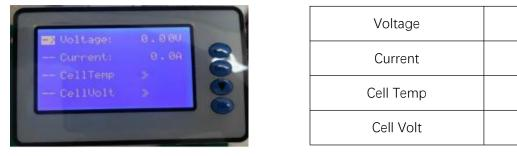
Move the cursor to "Cell Temp" and press "Enter" to check the battery temperature information, then press "  $\mathbf{\nabla}$ " to turn the page.
